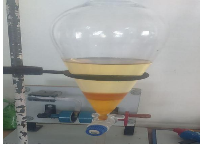
Biodiesel Distilled-Water Wash
